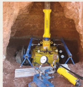
▲ In situ direct shear test, Tarlan complex
